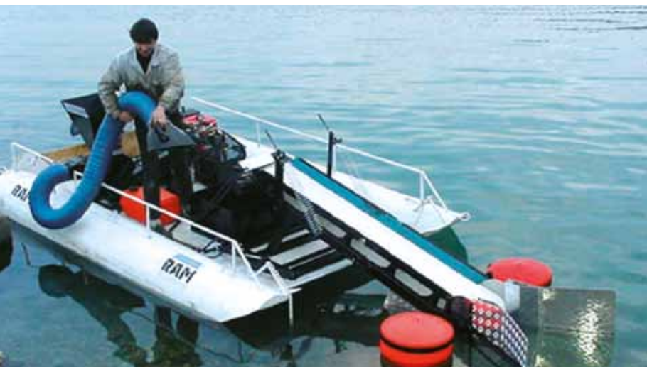
The antipollution boat lowers a magnetic drum in the sea to collect the 'CleanMag' material
