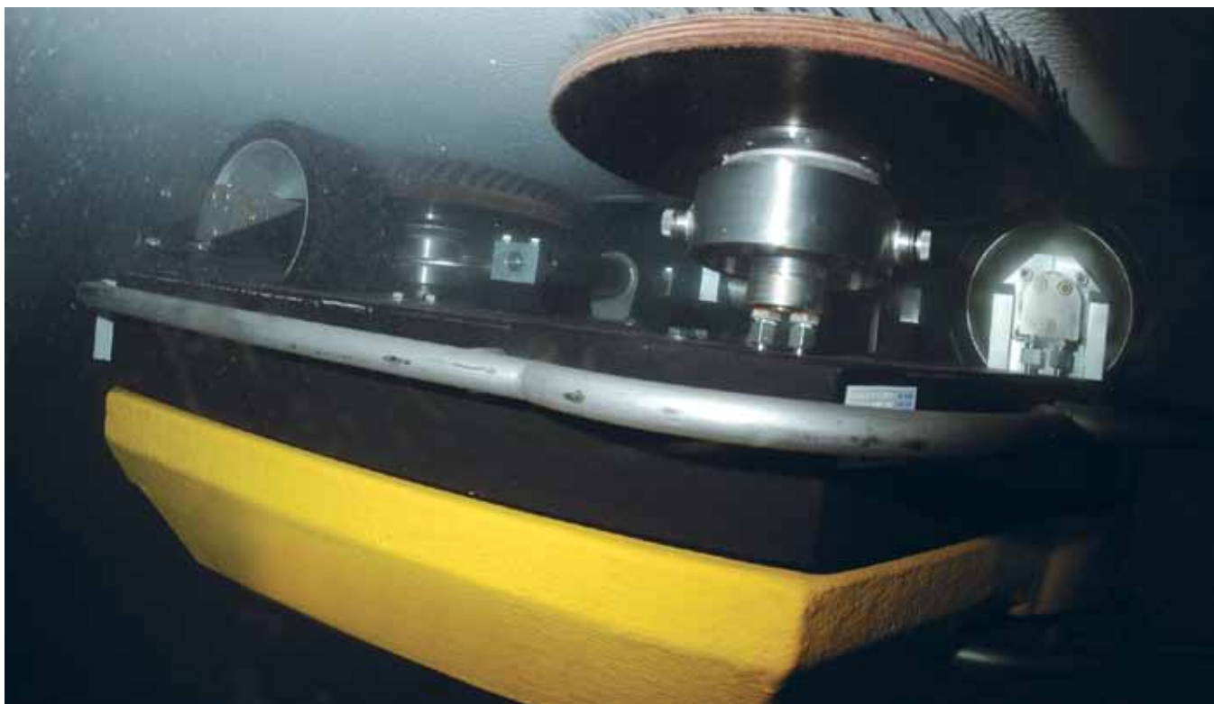
Regular underwater treatment using Ecospeed is a Best Available Technology to minimise the risk of transferring non-indigenous marine species
